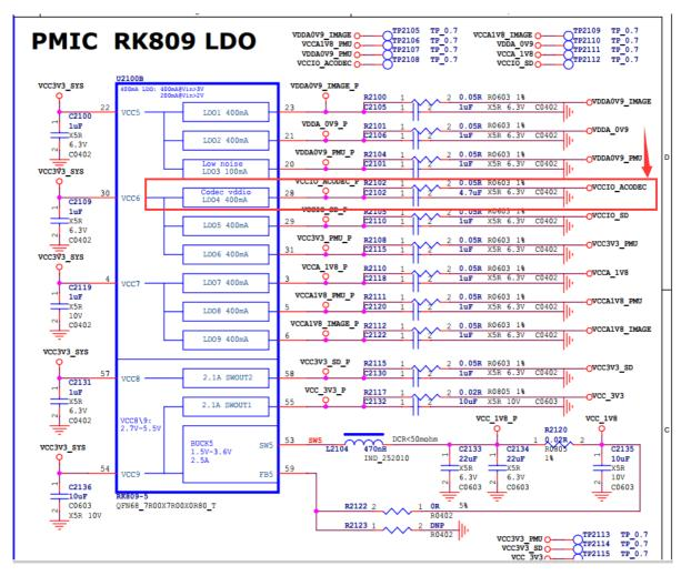
From the above figure, you will find that vccio\_acodec is powered by LDO4 of RK809. Find the configuration information of LDO REG4 (LDO4) from the dts file as follows:
