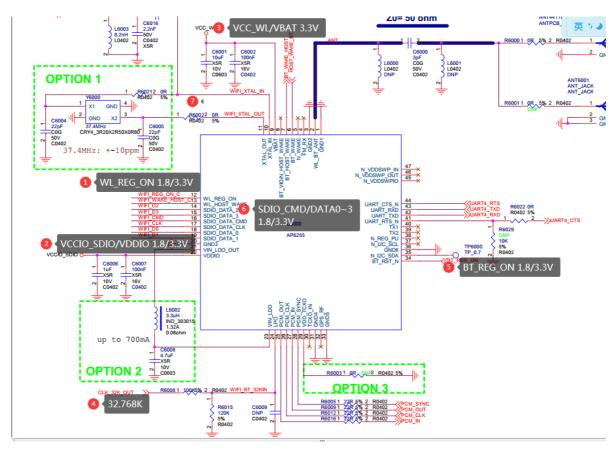
Use an oscilloscope to measure the timing of VBAT/VDDIO/WL\_REG\_ON and ensure it meets the following timing requirements:
