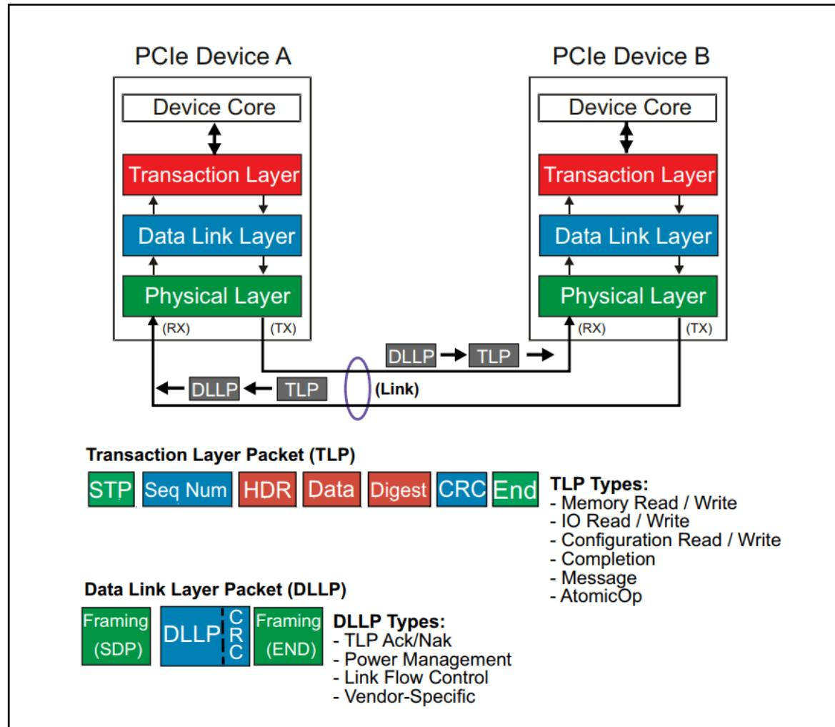
28 Byte TLP overhead 是冗余最大的传输包，包含 the header (16 bytes), the optional ECRC (4 bytes), the LCRC (4 bytes), the sequence number (2 bytes) and the framing Symbols STP and END (2 bytes).
